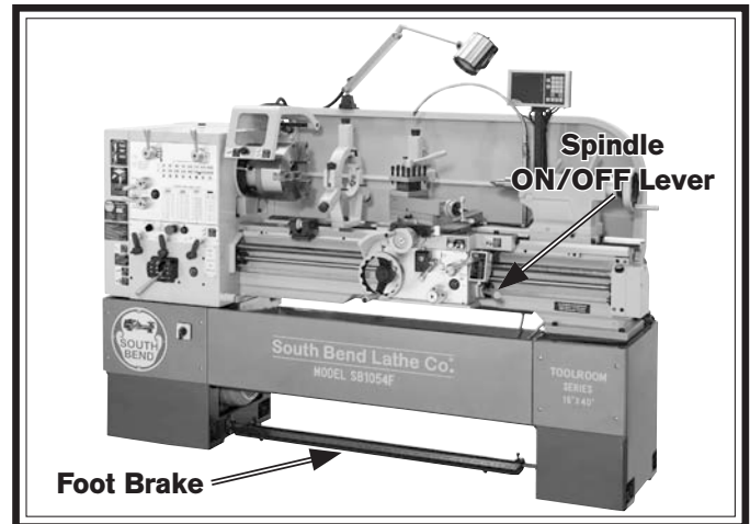
Figure 10. Foot brake and spindle ON/OFF lever.
